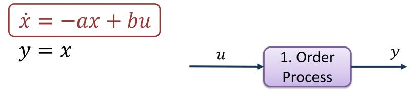
In order to simulate this model in LabVIEW you can make a discrete version of the model, or you can implement it as a "Block Diagram" using the features in LabVIEW Control Design and Simulation Module
